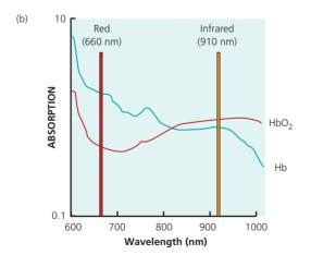
Figure 11.3 Pulse oximetry
