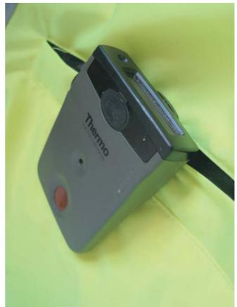
Figure 3.10 Electronic personal dosimeter.
