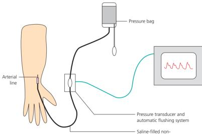
**Figure 11.7** Invasive blood pressure measurement. (Source: http://www.aic.cuhk.edu.hk/web8/haemodynamic %20monitoring%20intro.htm).
